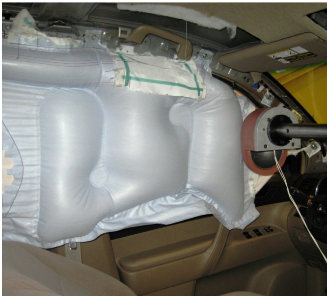
Figure 6: Curtain Air Bag (Wide Span)
